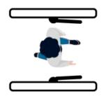
In case of a power outage, swing arms are unlocked and open automatically.
